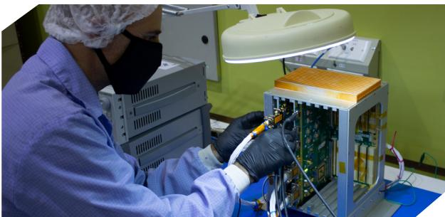
It has a power module, a Single Board Computer module based on the UT699 LEON3-FT 32-bit processor and 6 additional functional modules, all linked through the cPCI 2.2 standard through the use of a Backplane. It also has an additional slot, designed to adapt to the needs of different missions/projects.
